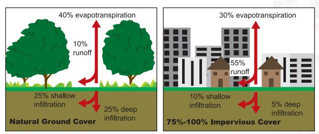
**Figure 1.** Relationship between impervious cover and surface runoff. Impervious cover in a watershed results in increased surface runoff. As little as 10 percent impervious cover in a watershed can result in water-quality problems. (Source: USEPA)
